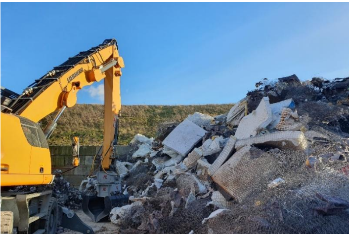
4 Machinery separating upholstery from mattress frames at Hamilton Waste and Recycling East Lothian, where much of the household waste from the Edinburgh Campus is processed
