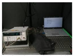
Fig 2. The actual set-up recording data in the lab. As you can see, the count rate is displayed on the frequency counter whilst the blackout sheet is covering the photon detector to record a dark count rate.
