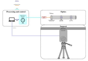
Fig 4. The complete set-up with the Agilent device and laptop controller as part of the full system consisting of a photon detector placed on a sweeping controlled platform.
