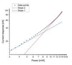
Fig 1. The current response of a silicon photodiode as the incident power is increased. The TPA data is displayed as a log-log plot, where the blue line is of slope 1, indicating SPA, and the red line has a slope of 2 representing TPA. show SPA at lower powers and then transition to TPA, an example of one experimental result can be seen in figure 1.
